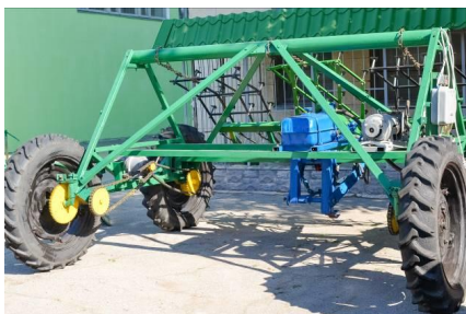
Fig. 1. Wide span vehicle design of the Tavria State Agrotechnological University (TSAU)
