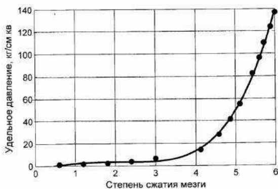
Figure 1 Dependence of the specific pressure in the pulp of castor seeds on its compression ratio
